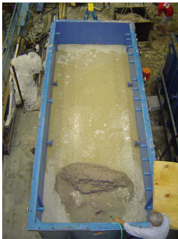
Figure 12.13. One of the Experimental Controlled Release System tanks being filled prior to the experiment. Photograph provided courtesy of C. Herb Ward, Rice University, Houston, Texas.
