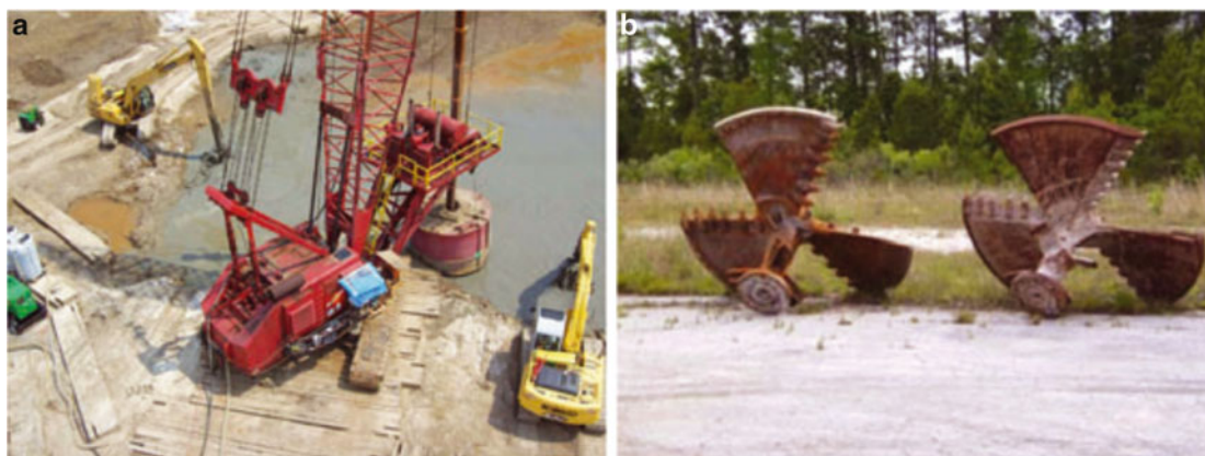
Figure 10.11. Apparatus used for ISSM at Camp Lejeune, NC. (a) Crane-mounted rotary table and hollow kelly bar, (b) 3.0 m diameter augers. From Olsen et al. (2012), used with permission.
