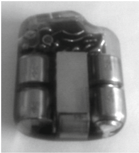
Fig. 1.2 Epoxy resin pacemaker
