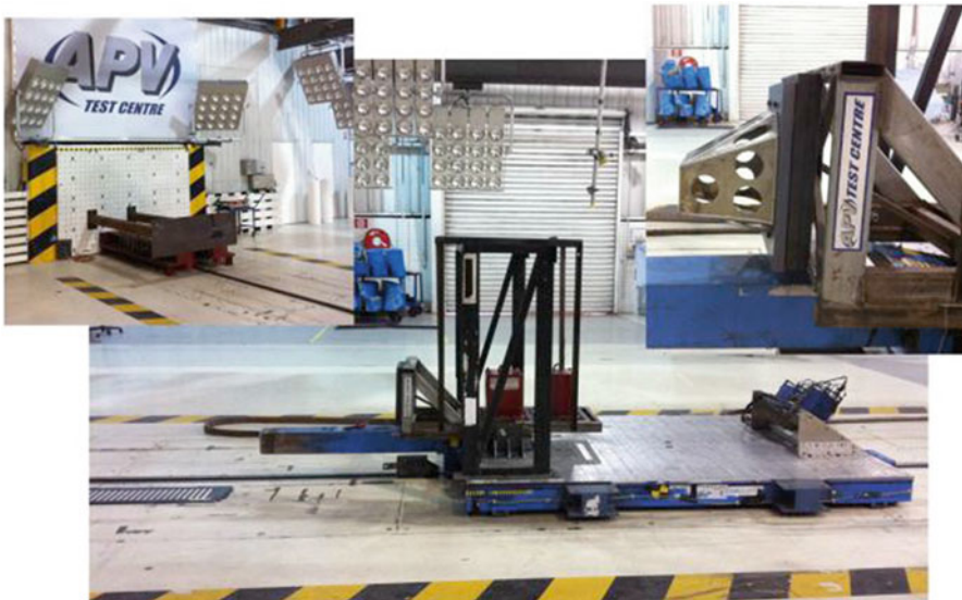
Fig. 7.6 The sled apparatus used in the crash test
