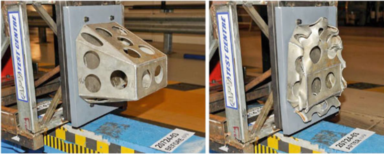
Fig. 7.7 The impact attenuator before and after the crash testing
