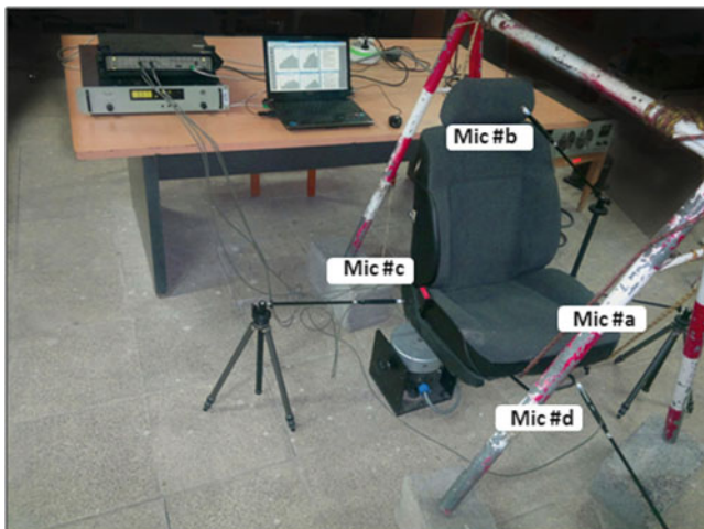
Fig. 8.17 Test setup and four selected points for measuring the sound pressure level
