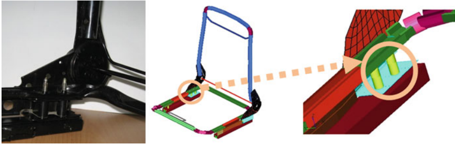
Fig. 8.11 Physical and finite element model of the seat, rails and structure conjunction is conducted via RBE element
