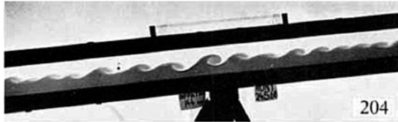
Fig. 6.2 A depiction of the Kelvin–Helmholtz instability between two fluids of different densities. The shear layer perturbations can be seen between the dark and light fluids [45]
