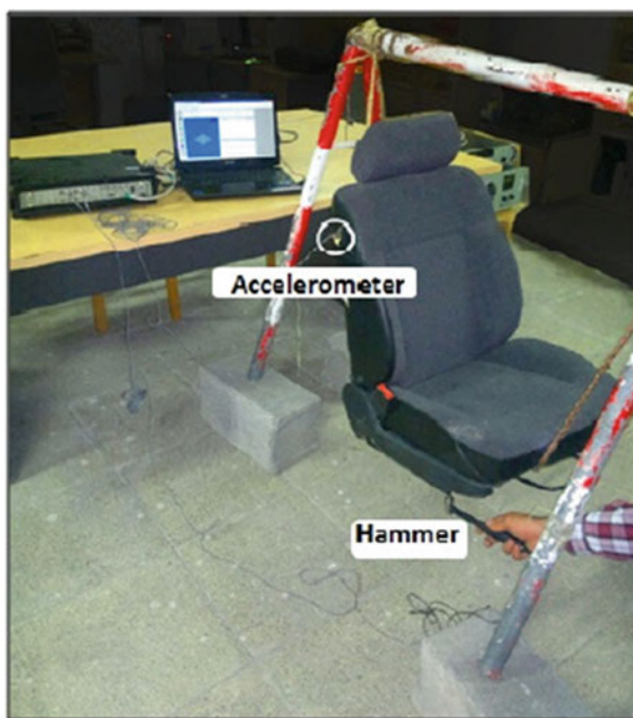
Fig. 8.12 Test setup to obtain modal characteristic of the seat
