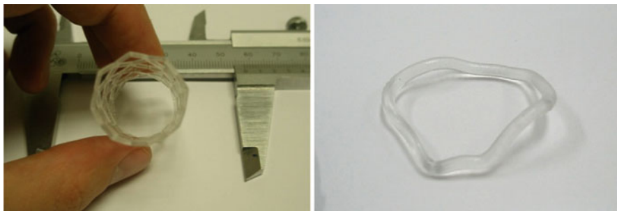
Fig. 10.4 Left image: prototype of stent in shape-memory epoxy. Right image: prototype of annuloplasty ring in shape-memory epoxy (Manufactured using laser stereolithography: SLA-3500 Machine 3D Systems)
