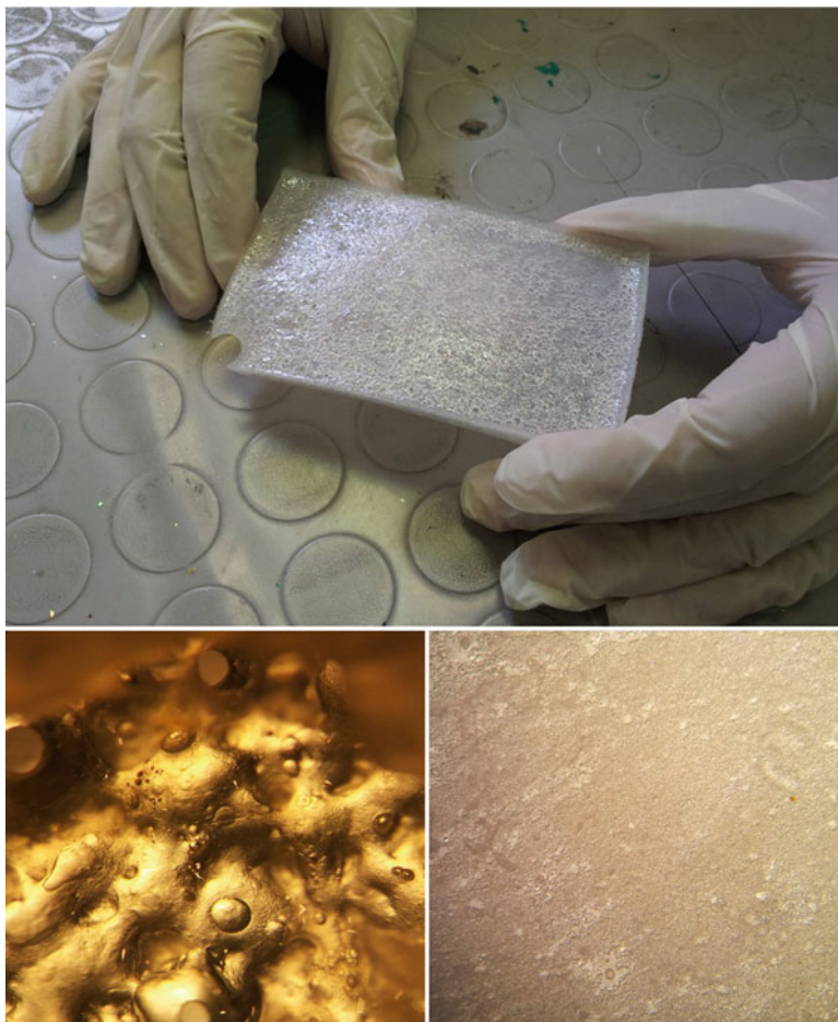
Fig. 12.8 Foam and emulsion obtained by mixing photopolymer (epoxy resin) and water. Microstructures obtained after UV polymerization and drying. Foam leads to pore sizes around 300–500 \mu\text{m} ( lower left image ) and emulsion leads to pore sizes around 30–50 \mu\text{m} ( lower right image )
