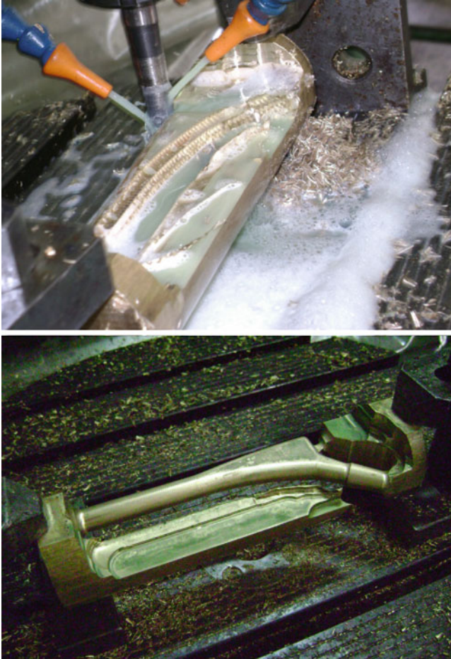
Fig. 9.4 CAM-assisted CNC machining of artificial hip prosthesis
