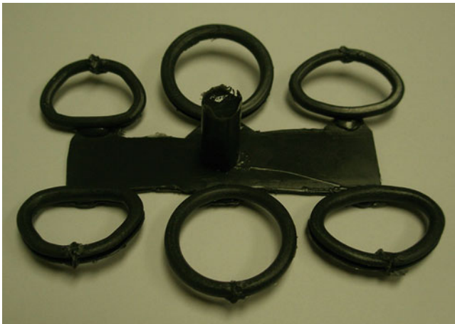
Fig. 11.4 Active annuloplasty rings manufactured by vacuum casting in silicone mould using shape-memory polyurethane with graphite powder (12 % weight)
