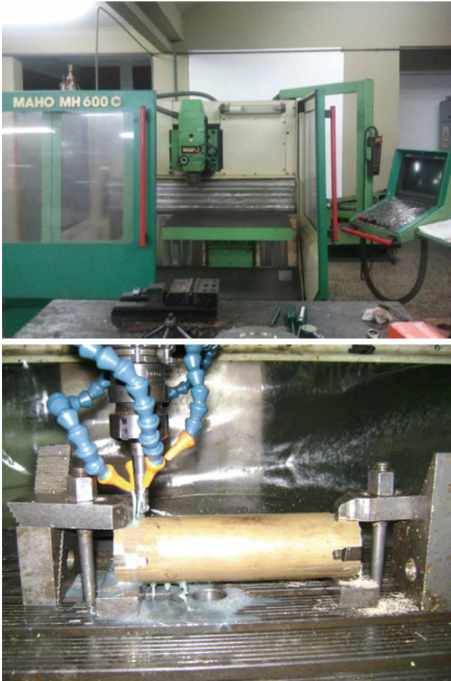
Fig. 9.3 CAM-assisted CNC machining of artificial hip prosthesis
