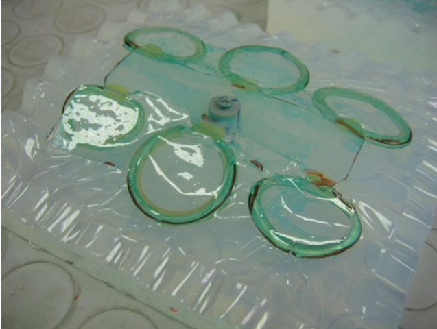
Fig. 11.2 Silicon mould. Aspect after cutting and separation of the two mould cavities, just before extraction of the model for subsequent casting
