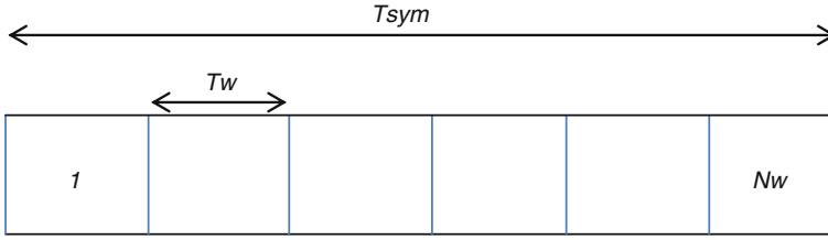
Fig. 4.14 The symbol structure for DBPSK/DQPSK impulse radio
