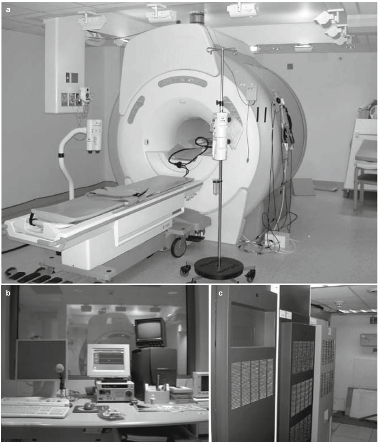
Fig. 13.1 Composite photograph of major components of a typical MRI system. (a) Scanner magnet and patient table; the table accommodates patient entry, exit, and positioning within the magnet bore. (b) Operator's console, which is remote from the scanner, allows control of
