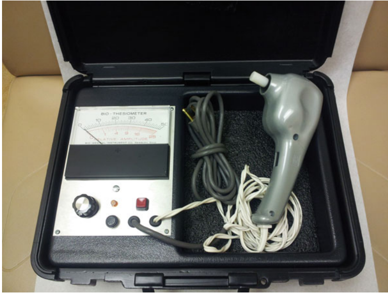
Fig. 19.1 The biothesiometer is an instrument designed to measure simply and accurately the threshold of appreciation of vibration in human subjects ( http://www.biothesiometer.com )
