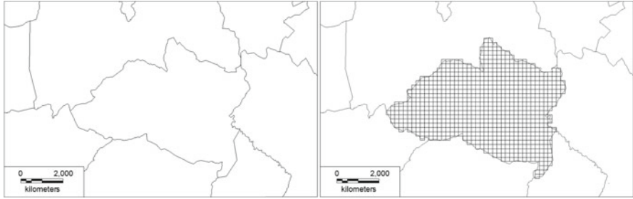
Fig. 8.1 Difference between vector-based GIS and raster-based GIS. Left: A parish map with one of the parishes highlighted. Right: The same parish in 250×250 m raster cells. The large cell size is used here for illustration. Smaller cells would obviously give a better outline of the area
