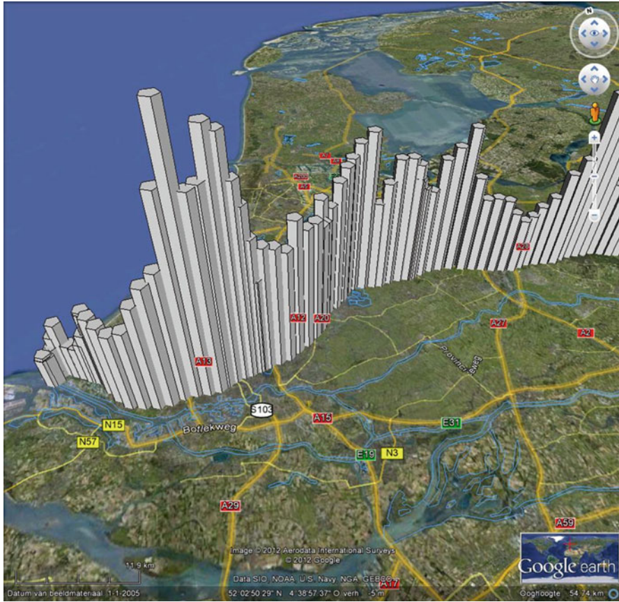
Fig. 9.13 Air pollution exposure along a GPS track. The height of the columns indicates the air pollution concentration
