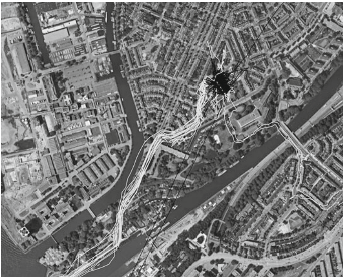
Fig. 9.4 GPS track where indoor ( black ) and outdoor ( light ) segments are differentiated, based on a filter (see Textbox 9.1)
