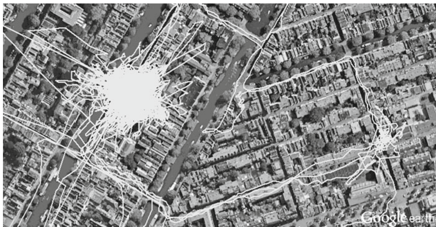
Fig. 9.2 Raw GPS track data, shown on a map. This example shows two typical clusters of “bad data” as recorded while the receiver is inside a building
