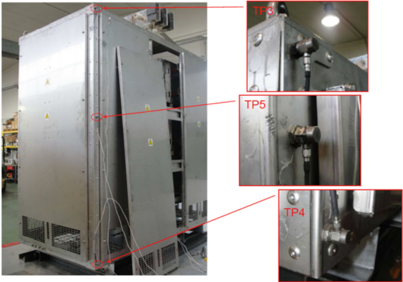
Fig. 37.6 Measuring points for the transverse test (part 1)
