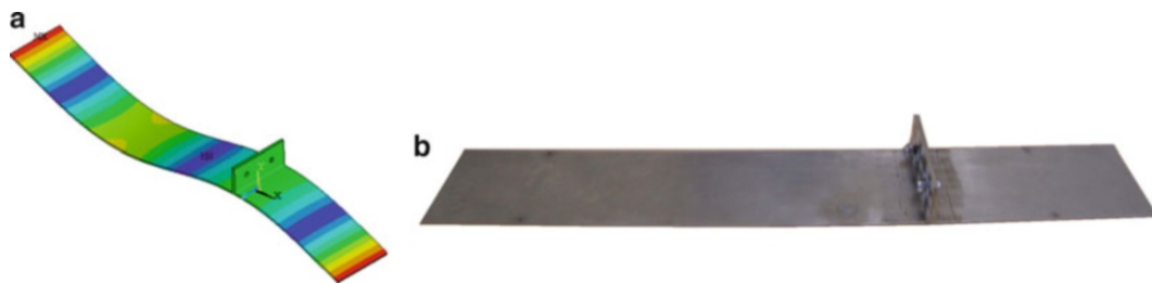
Fig. 14.2 Second bending mode of the flange model (a), and manufactured test piece (b)
