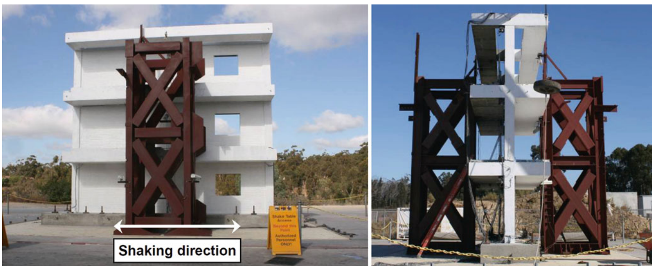
Fig. 7.1 Three-story test structure on the UCSD-NEES shake table
