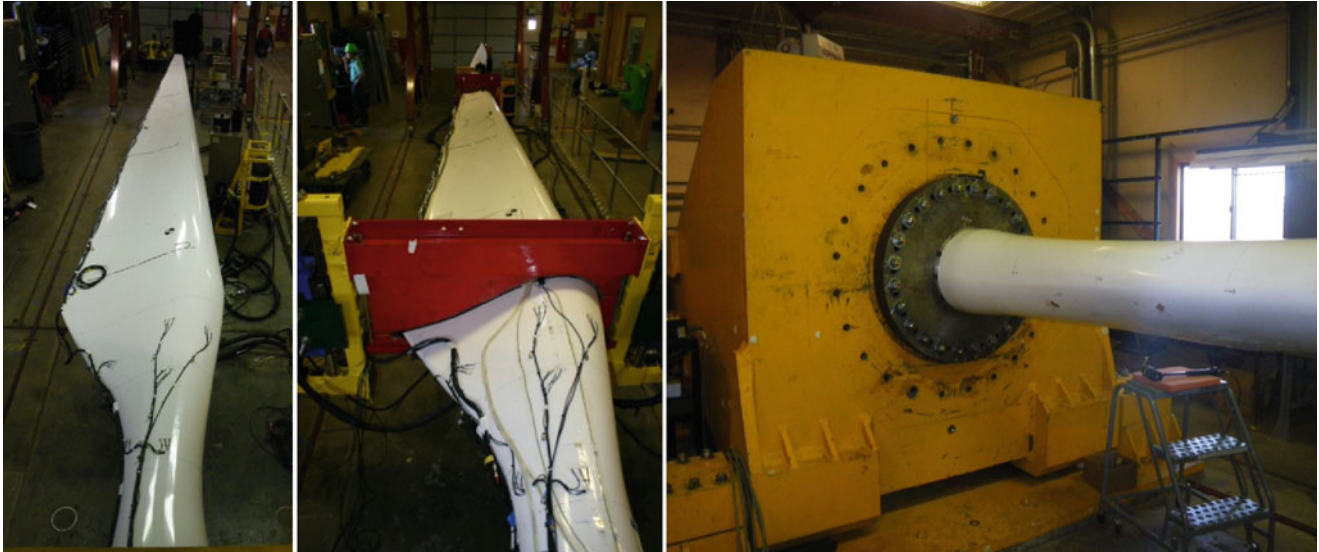
Fig. 11.2 Experimental fixed-free ( left ) configuration, mass-added ( middle ) configuration, and base fixture ( right )
