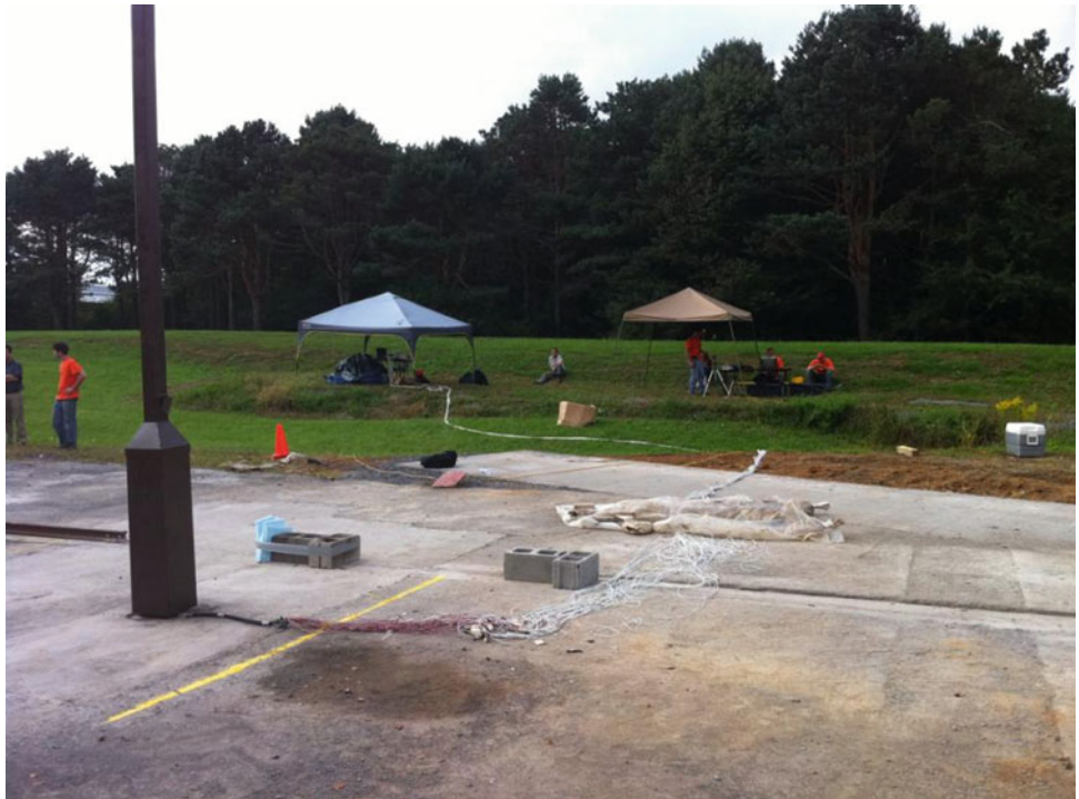
Fig. 15.3 Data acquisition system and lamp post ready for crash testing
