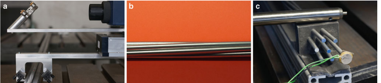
Fig. 18.4 Experimental setup for the investigation of wave propagation in coupled cylindrical waveguides using a Laser Doppler Vibrometer. Mirrors are used to measure radial velocities from the top and both sides. (a) Vibrometer and mirror setup. (b) Seven-rod structure. (c) Wave excitation with piezo
