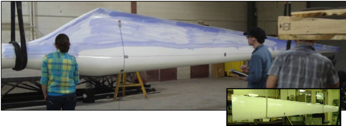
Fig. JH-11 Test setup of entire blade as well as only tip section, both in free-free configurations
