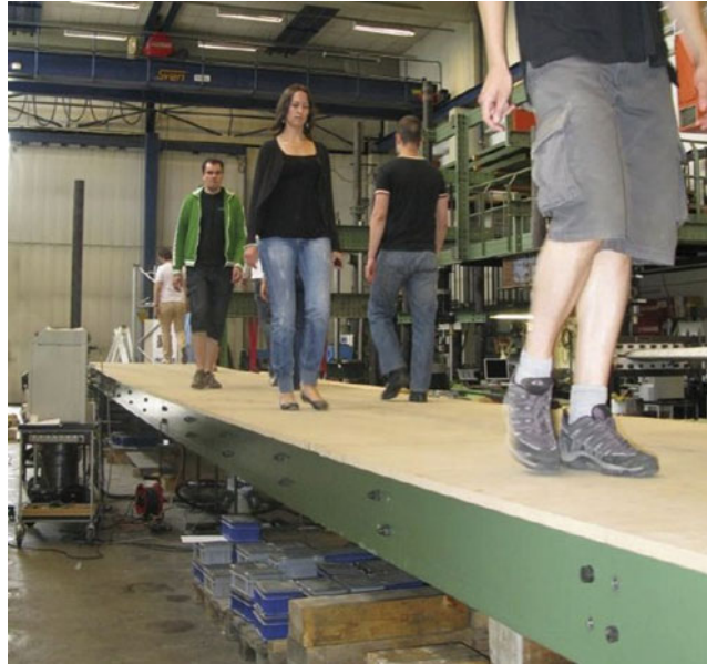
Fig. 4.2 Pedestrians traversing the 16 m long DTU laboratory footbridge
