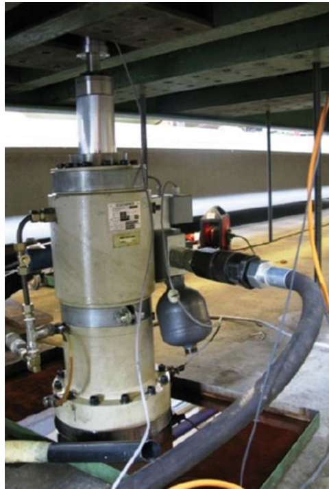
Fig. 4.3 Actuator at footbridge mid-span with hinged load cell
