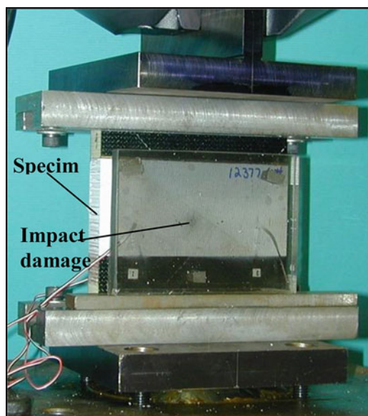
Fig. 1.23 Edgewise compression test on an impact-damaged sandwich panel
