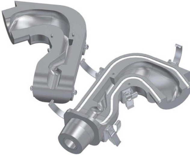
Fig. 12.9 “Alberta” idealized adult anatomic throat (AIT) commercialized by Copley Scientific Ltd, as inlet to an NGI ( Courtesy of Copley Scientific Ltd )
