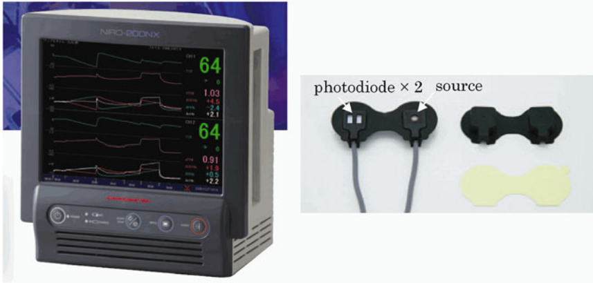
Fig. 1.8 Spatially resolved spectroscopy system (NIRO-200NX) with an optical probe consisting of photodiodes and a light source
