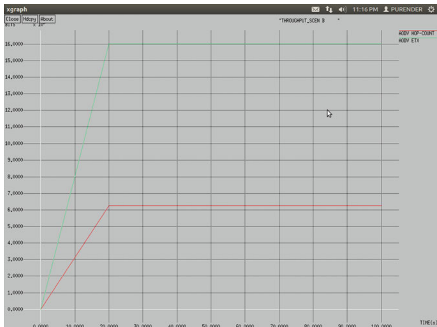
Fig. 3 Throughput for ETX versus Hop-Count metrics in Scenario B
