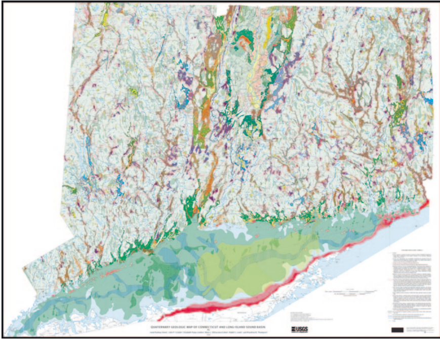
Fig. 2.6 A digital image of sheet one of the Quaternary Geologic Map of Connecticut and LIS Basin (Stone et al. 2005). The LIS Basin portion of this 1:125,000-scale map is a compilation of information from individual maps (such as the sampling shown on Fig. 2.5) and other sub-sea-floor data collected as part of the GHNS/USGS Cooperative Mapping Program. Image courtesy of Janet R. Stone
