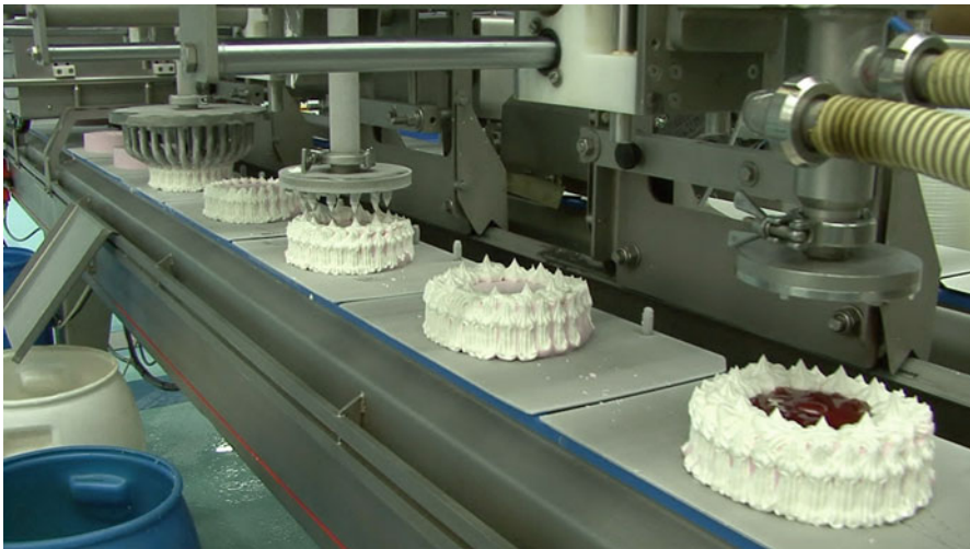
Fig. 9.22 Vertical extrusion and decoration of ice cream cakes on an automated line (courtesy Gram Equipment of America, Tampa, FL, USA)
