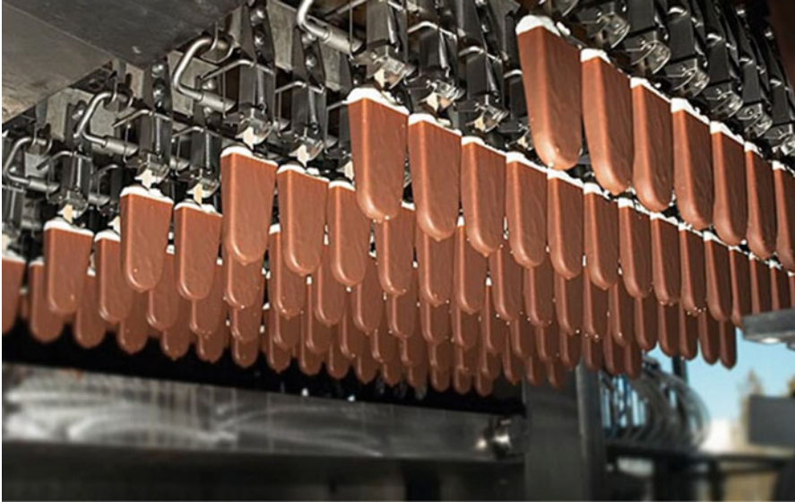
Fig. 9.11 The coating of ice cream bars in a thermostatically controlled dip tank
