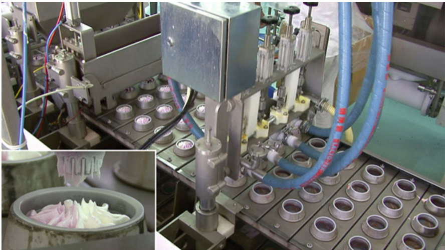
Fig. 10.8 Cup filler with multiple flavors depositing on parallel lanes. Inset shows details of filling station (courtesy of Gram Equipment of America Inc., Tampa, FL)
