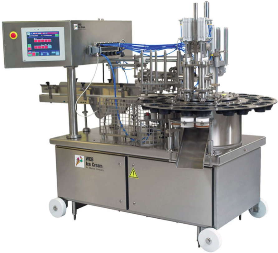
Fig. 10.6 Dual-lane rotary type filler for cups and round nested containers (courtesy of WCB Ice Cream, Northvale, NJ)
