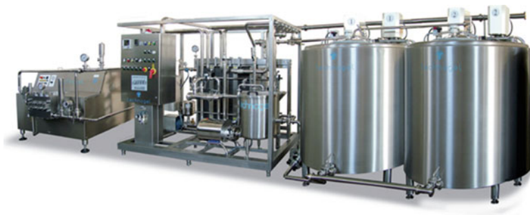
Fig. 5.9 Complete mix processing plant for small to mid-size operations, 600–5,000 L/h, including blending tanks, HTST pasteurization, homogenization, plate cooling, and aging tanks (courtesy of Technogel, Bergamo, Italy)
