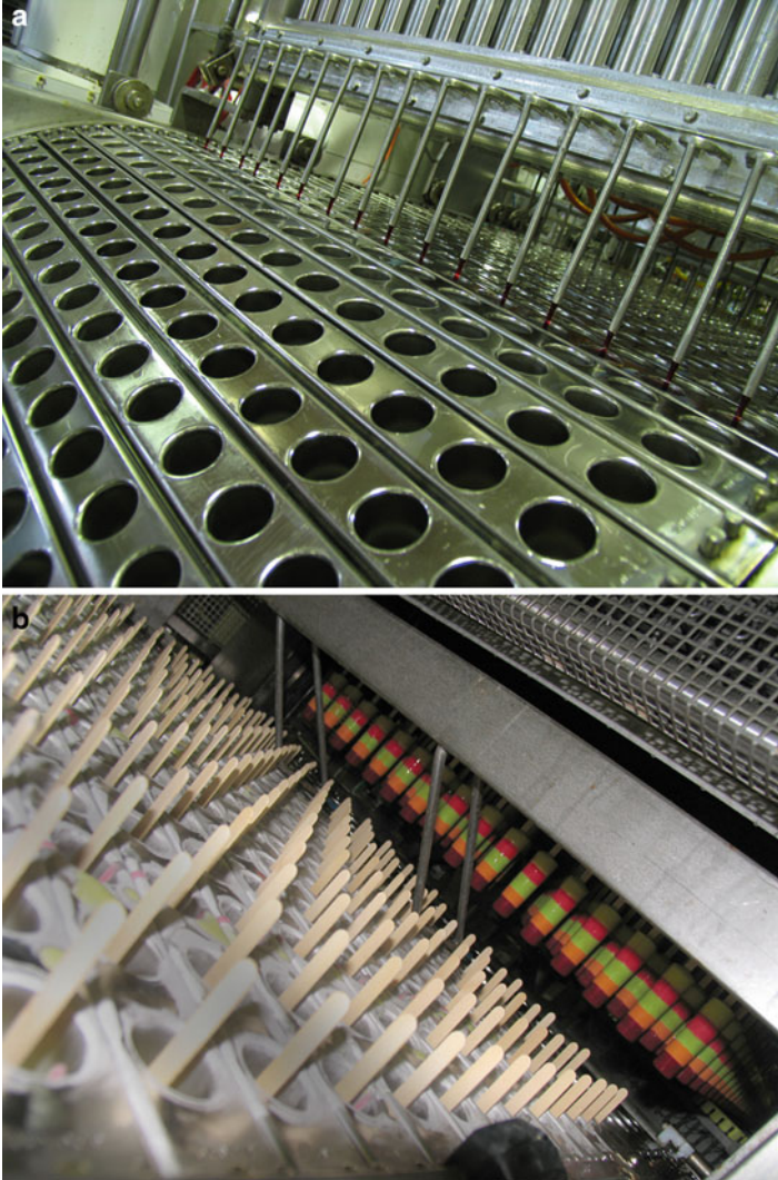
Fig. 9.8 Filling of a water ice mix into molds (a) and extraction of a multilayer water ice product from molds (b) on an in-line or straight-through molding machine (Gram Polo, courtesy of Gram Equipment of America, Tampa, FL, USA)
