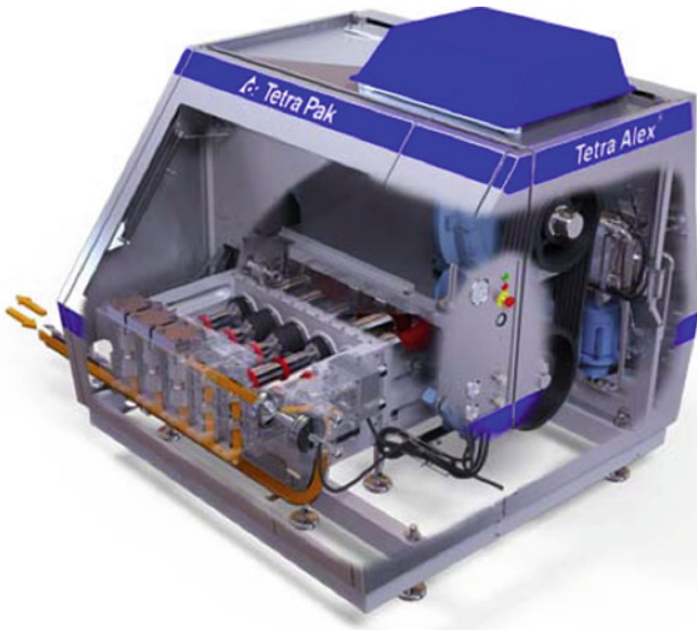
Fig. 5.10 Industrial five-piston homogenizer (TetraPak Alex), showing flow through the piston pump. The homogenizing valve assembly sits at the exit of the pump (courtesy of TetraPak Hoyer A/S, Høebjerg, DK)
