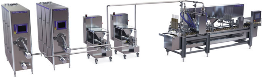
Fig. 10.3 Sequence of freezing, ingredient addition, and filling (courtesy of Tetra Pak Hoyer A/S, Høejbjerg, DK)
