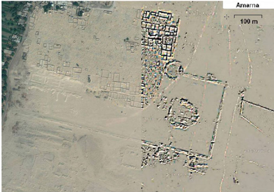
Fig. 6.8 The Temple of Amarna, Egypt as seen on Google Earth imagery ( left ). The right half of the image has had contrast stretch applied to bring out details related to man-made structures
