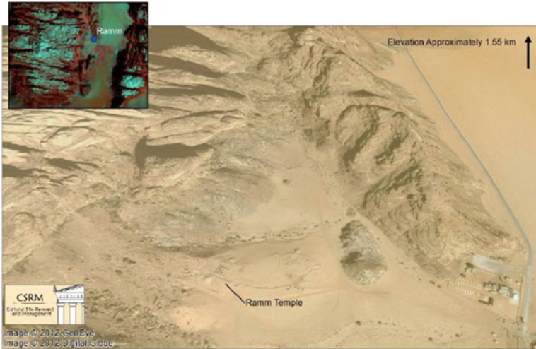
Fig. 7.6 Oblique view of Nabataean temple (Ramm) in Google Earth. Inset is an NDVI image, showing temple in spatial relation to arable soils (seen as red in NDVI) and rock slopes that channel water to arable soils, making agriculture possible
