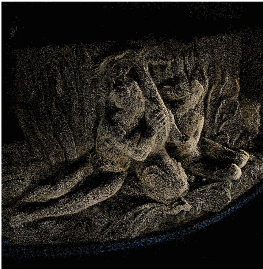
Fig. 14.1 A colorized point cloud representation of a fountain at the Santa Barbara County Courthouse, created by Photosynth™ website user EdLee
