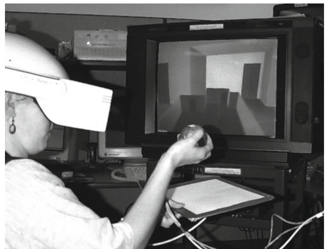
Fig. 28.2 Immersive VR system. The WIM graphics attached to the clipboard are a miniature copy of all the surrounding graphics in the immersive environment. Each of the objects in the WIM copy is tied to their counterparts in the immersive environment through pointers and vice versa at the point of WIM creation. The user can manipulate the objects in the WIM, and the objects in the world will follow (Reprinted from Stoakley et al. [19]. With permission ACM Press/Addison-Wesley Publishing Co.)
