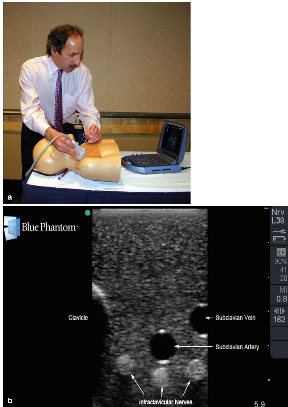
Fig. 34.2 (a) “Ultrasound Andy,” the original Blue Phantom™ head-neck-upper torso ultrasound-guided regional anesthesia and central venous access model. (b) Ultrasound image of “Ultrasound Andy’s” infraclavicular brachial plexus (Reproduced with permission from Blue Phantom™, Redmond, VA)
