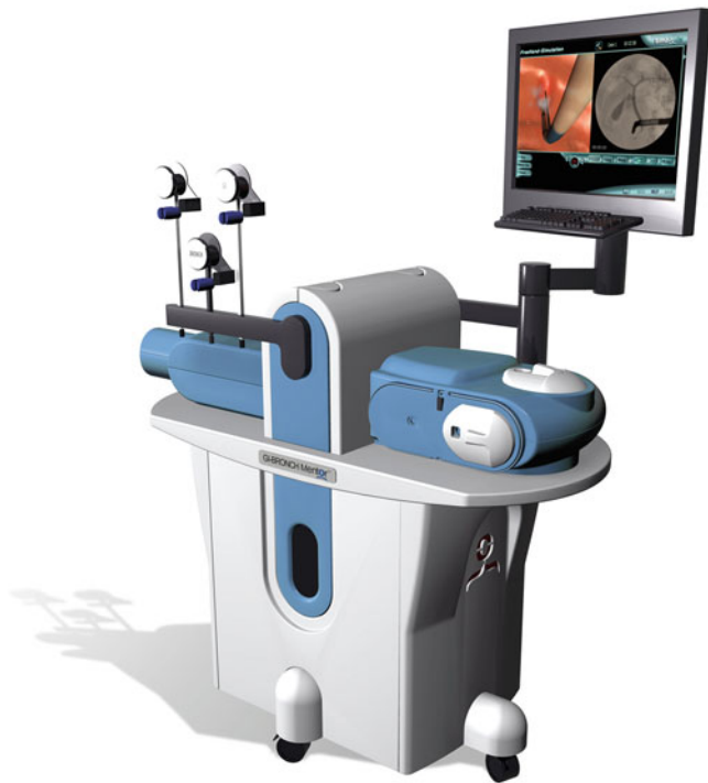
Fig. 24.5 Symbionix's GI Mentor is a virtual reality model for computer-based part-task endoscopic simulation. A modified endoscope can be inserted through one of the mannequin's two orifices while projecting the examination onto a monitor (Image used with permission from Symbionix)
