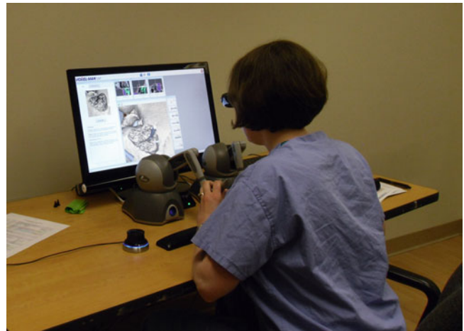
Fig. 33.2 Virtual reality temporal bone simulator (VOXEL-Man, Hamburg, Germany), providing auditory information, haptic interface, and metrics
