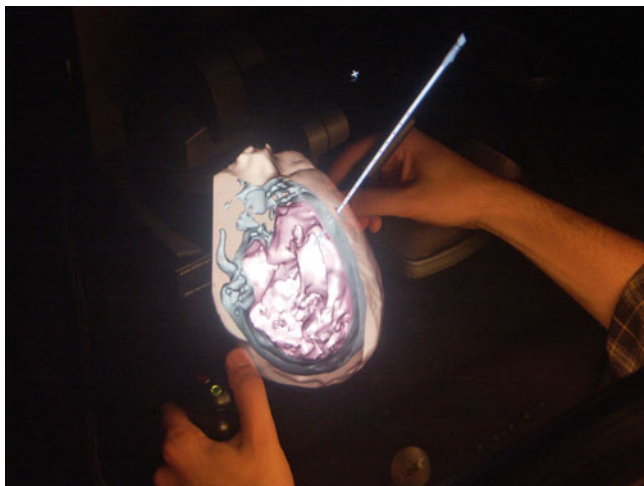
Fig. 28.5 A ventriculostomy simulation. The trainee is inserting the ventricular catheter according to skull landmarks. A virtual cranial window is shown to check the location of the tip of the ventricular catheter (Image courtesy of ImmersiveTouch)
