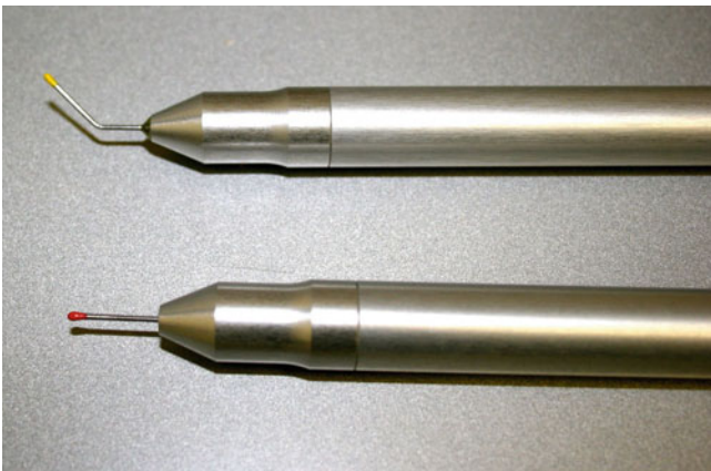
Fig. 31.5 Examples of the “handpieces” of the Eyesi® simulator. Once placed through one of the ports of the model eye, the instrument will appear as the needed instrument for the task i.e., capsulorhexis forceps, irrigation cannula, and phacoemulsification hand piece
