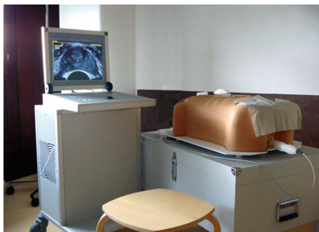
Fig. 25.2 TRUS simulator (MedCom, Germany). This virtual simulator allows the learner to place an ultrasound probe in a simulated rectum and practice coronal and axial viewing of the prostate
