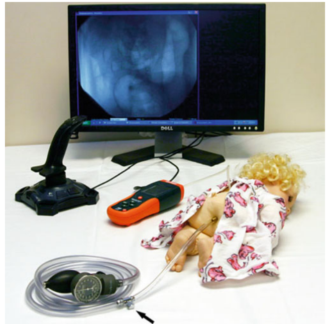
Fig. 38.8 Photograph of a simulator created for practicing intussusception reduction. Plastic tubing with the external release valve ( arrow ) connects the aneroid gauge and bulb insufflator to the cylinder within the doll. Additional tubing extends from the doll to a pressure sensor and is transmitted via USB cable to a computer. The computer displays simulated images taken during an intussusception reduction (Reprinted from Stein-Wexler et al. [43], with permission from Springer)
