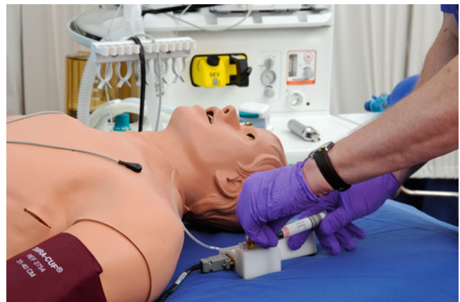
Fig. 15.13 METI HPS® Human Patient Simulator drug recognition system uses barcode technology to accurately identify drug administered, concentration, and dose (Photo courtesy of CAE Healthcare ©2012 CAE Healthcare)
