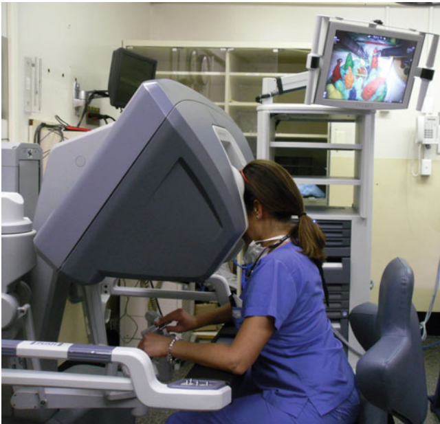
Fig. 33.7 Learner at a robotic console (da Vinci, Intuitive, Sunnyvale, CA), demonstrating practice of robotic manipulation skills with nonanatomic tasks
