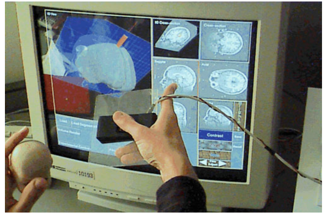
Fig. 28.1 The simulator interface allows neurosurgeons to explore a 3D MRI scan of a patient's brain during presurgical planning. From the surgeon's perspective, the interface is analogous to holding a miniature head in one hand which can be "sliced open" or "pointed to" using a cross-sectioning plane or a stylus tool, respectively, held in the other hand (Reprinted from Publication Hinckley et al. [17]. With permission from IOS Press)
