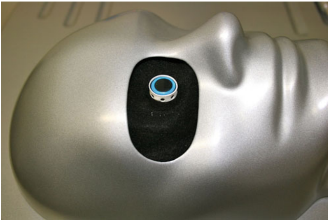
Fig. 31.4 The Eyesi® simulated patient and eye. Each of the ports on the outer aspect of the eye will allow for placement of one of the system's instruments
