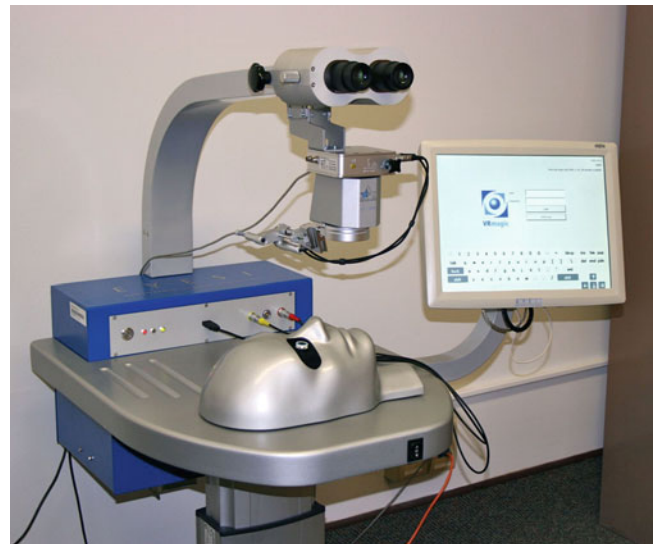
Fig. 31.3 The Eyesi® simulator. The system has oculars and operating scope model. The adjacent monitor will project the same view as the participant views through the ocular. There are two foot pedals designed in a similar fashion to the operating scope: foot pedal and the phacoemulsification machine pedal. The head can be positioned so that the operator can sit either temporally or superiorly
