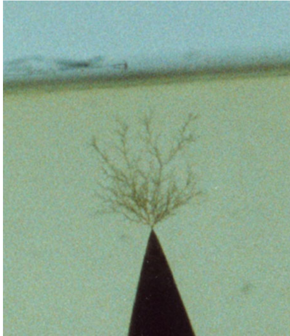
Fig. 7.6 An electrical tree grown in epoxy resin
