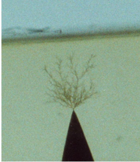
Fig. 7.6 An electrical tree grown in epoxy resin
