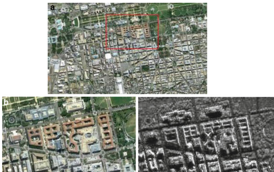
Fig. 2.1 Data set 1—SAR image of 306 \times 350 pixels. (a) original optical image of Washington and (b) the first applied SAR image obtained from the original image and its comparative optical image
