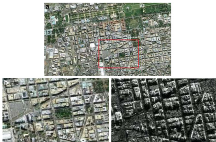
Fig. 2.2 Data set 2—SAR image of 93 \times 121 pixels. (a) original optical image of Washington and (b) the second SAR applied image obtained from the original image and its comparative optical image
