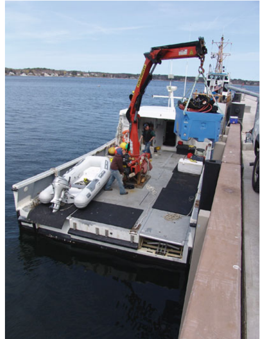
Mussel Culture, Open Ocean Innovations. Figure 4 A hydraulic articulating crane on a service vessel, shown here being used to unload equipment, is used extensively in mussel farming operations
