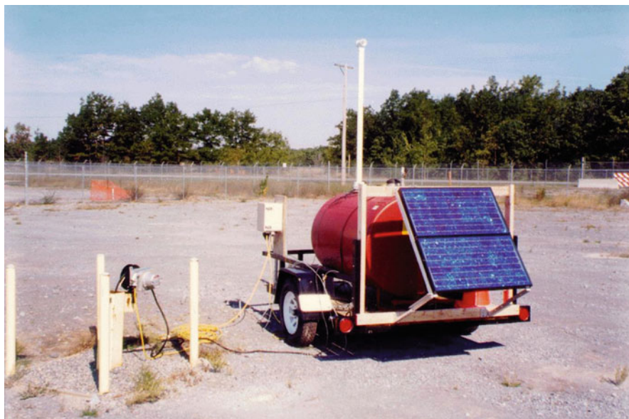
Fig. 13.2 Example of solar powered system with photovoltaic panels for powering product skimming
