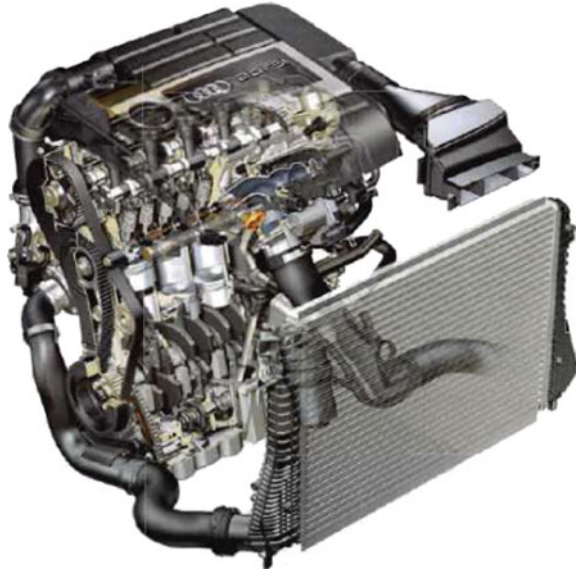
Fig. 6.3 Illustration of the Audi 2.0-L TSI, an example of an in-line four-cylinder engine (Used with permission from [4])
