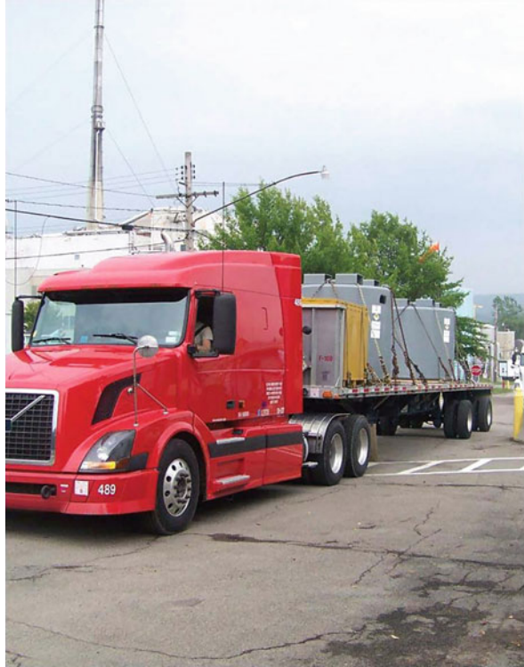
Fig. 9.9 Low-level radioactive waste packages for offsite disposal [42]
