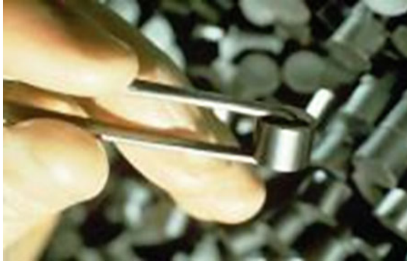
Fig. 7.1 Uranium dioxide ( \text{UO}_2 ) fuel pellet (Courtesy AREVA)
