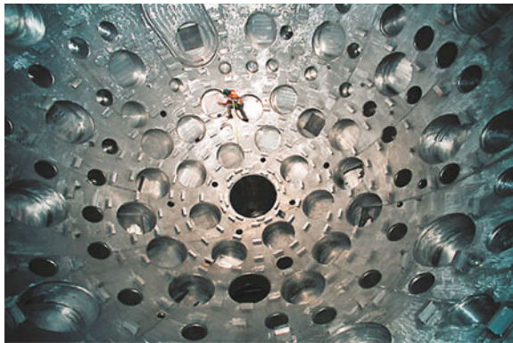
Fig. 12.25 The NIF target chamber, with holes where the laser beams enter. (The wide angle photo makes the 10-m diameter chamber appear to be larger.) (Courtesy of Lawrence Livermore National Laboratory)
