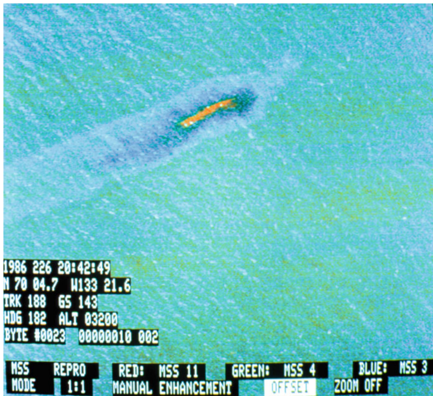
Fig. 15.9 A test slick highlighted using overlaid infrared and visible imagery. This results in a very relative “thickness map” of this particular slick. This technique is not particularly useful for most slicks as they do not show this gradient, which is only typical for small, recently spilled slicks
