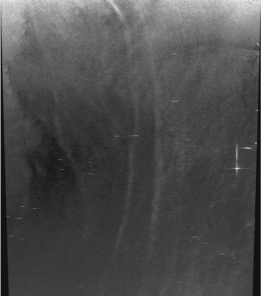
Fig. 15.17 A VV polarized view of the same area of sea surface. Note that this polarization yields a slightly clearer image of sea surface details than that shown in Fig. 15.16
