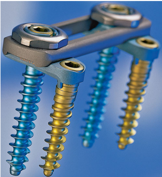
Fig. 21.1 MACS-TL® plating system. The blue polyaxial screw is connected to a clamping element through which the yellow stabilization screw is inserted. A plate connects both clamping elements (Copyright Aesculap Implant Systems, LLC; used with permission)
