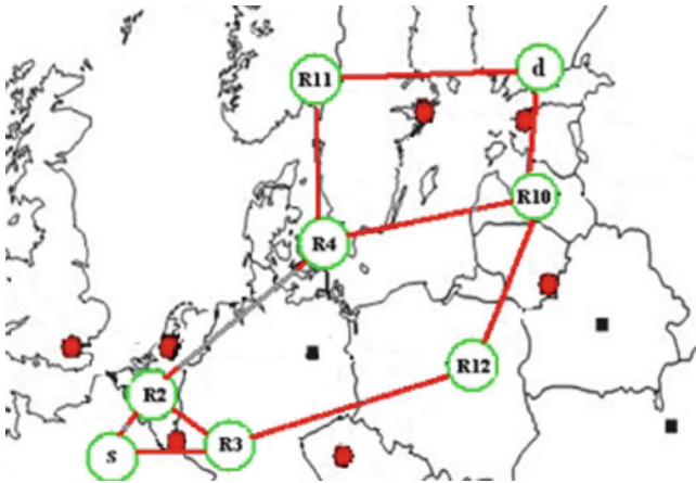
Fig. 5.8 The virtual topology G(s, d) , assuming regeneration sites R2, R3, R4, R10, R11, and R12. Source s and destination d are transparently connected to sites R2 and R3 and R10 and R11, respectively
