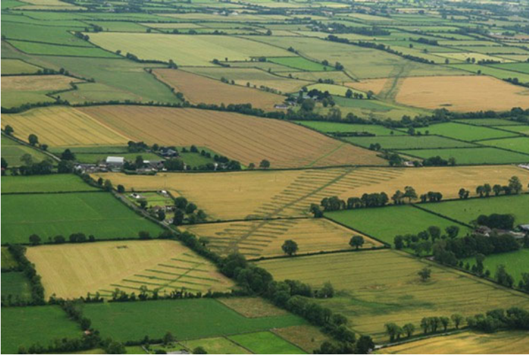
Fig. 15.3 Test trenching of proposed road corridor of N9/N10 Phase 4 Knocktopher to Powerstown, Co. Kilkenny, Ireland (courtesy of National Roads Authority)
