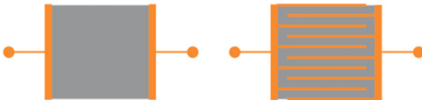
Fig. 16.4 The read-out of the resistance of metal-oxide layers may be hampered by its extremely high values. For a given area of active material, it turns out, by geometrical arguments, that interdigitated electrodes ( right ) are more effective than planar ones ( left )
