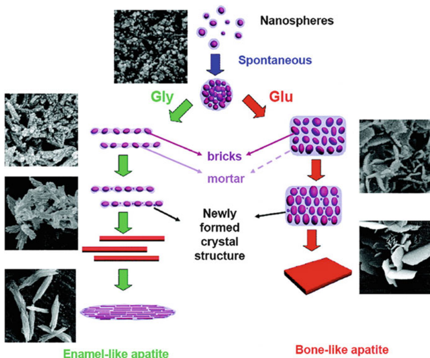
Fig. 4.4 Model of hierarchical assembly of apatite nanocrystals mediated by glycine and glutamic acid. Nanocrystals consisting of HAP core (purple) and ACP shell (light blue) aggregated spontaneously and were dispersed in water. In the presence of indicated amino acids, nanocrystals reassembled into different hierarchical structures. One-dimensional linear assemblies and two-dimensional plate-like structures were formed in the presence of Gly and Glu, respectively. Nanocrystals were connected by ACP surrounding HAP core. ACP transformed into thermodynamically stable HAP, and, at the same time, HAP core rotated to the most stable orientation. As a result, each HAP domain had the same crystallographic orientation and fused into single crystals. Reprinted with permission from [73]. (Copyright 2007, American Chemical Society)
