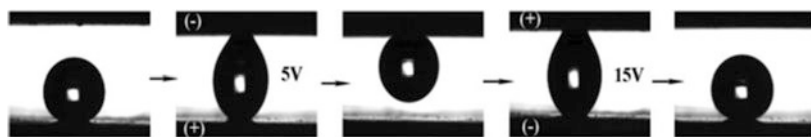
Fig. 9.12 Controllable pinning and transport of a nearly spherical water droplet between two superhydrophobic MTA membranes. Reprinted with permission from ref. [50]. Copyright (2011) Wiley-VCH
