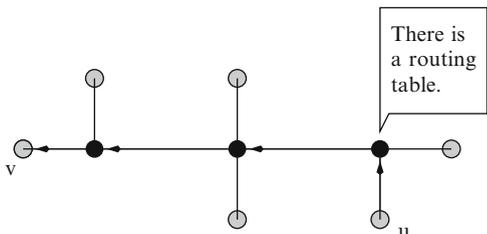
backbone is required to have two properties: (1) Every node not in virtual backbone should be able directly to communicate with (adjacent to) a node in the virtual backbone. (2) All nodes in the virtual backbone should be able to communicate each other within the virtual backbone, that is, the virtual backbone induces a connected subgraph.
