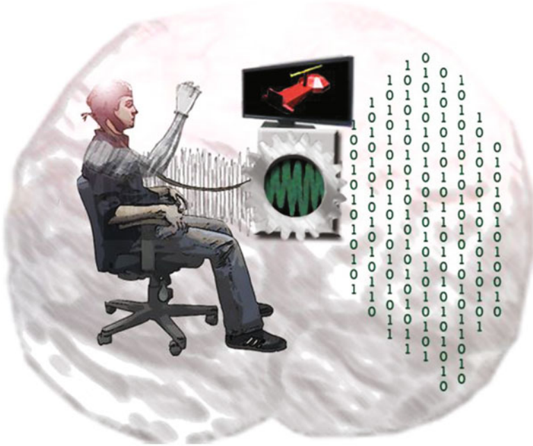
Fig. 2.7 A diagrammatic representation of an EEG-based BCI system. Using motor imagery paradigm, human subjects control the three-dimensional movement of a virtual helicopter. Raw EEG is temporally and spatially filtered to produce individualized control signal components. These components are weighted and digitized in a subject-specific manner and output to influence control in the virtual world (from [52], with permission)
