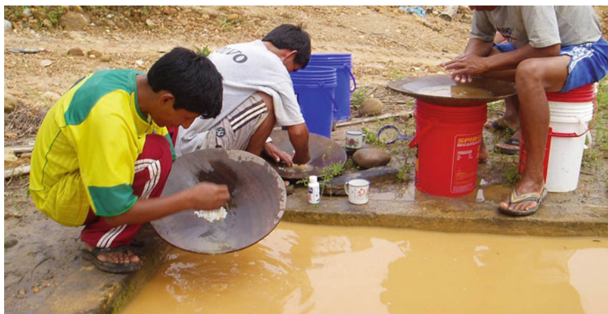
Fig. 10.3 Modern batea by small scale miners. Note silvery gold–mercury amalgam in the bottom of the batea and small white plastic bottle of mercury along the cement wall of the muddy tank
