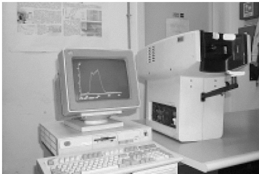
Fig. 14.6 QELS probe integrated with fluorometry measurements in a fluorotron master (Photo courtesy of Luigi Rovati, Ph.D., University of Modena)
