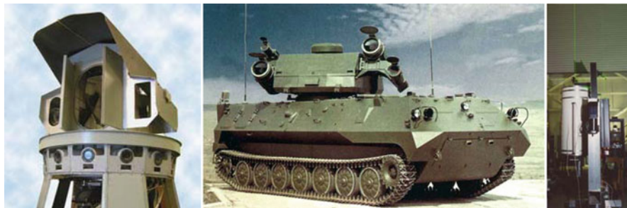
Fig. 10.1 Civilian, military, and scientific purpose lidars for atmosphere investigation (from left to right ): Lidar automatic system for remote air pollution monitoring in large industrial areas (Institute of Precision Instrumentation, Moscow); Laser system for remote chemical agents detection (Astrofizika Corp., Moscow); Raman lidar at the Pennsylvania State University
