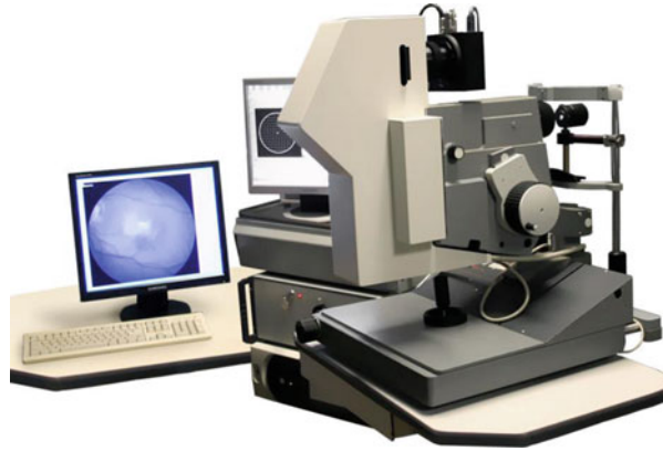
Fig. 11.17 General view of the multispectral fundus imager with adaptive compensation of human eye aberration
