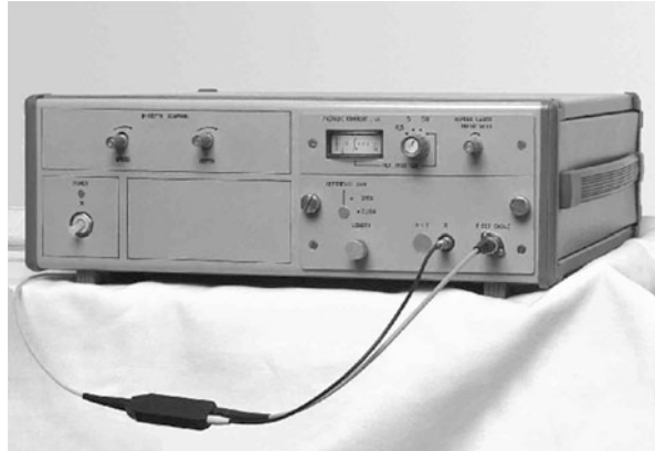
Fig. 24.4 General view of the portable optical coherence OCT device
