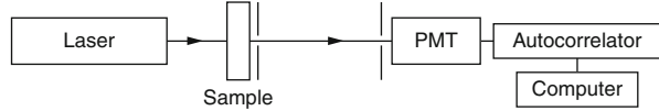
Fig. 1.11 Typical scheme of DWS experiment with use of the transmitted light detection
