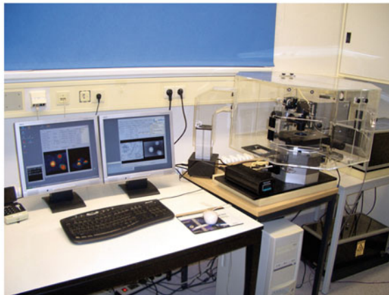
Fig. 6.2 Upper panel: schematic of the modular integration of digital holography into an inverted microscope (Modified from [23]), lower panel: photo of an experimental setup (iMIC, TiLL Photonics GmbH, Munich, Germany, modified for DHM) with included heating chamber (Solent Scientific Ltd., Segensworth, United Kingdom) for live cell imaging
