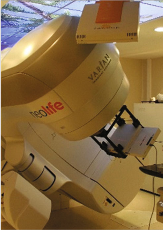
Fig. 20.4 Gantry mounted array
