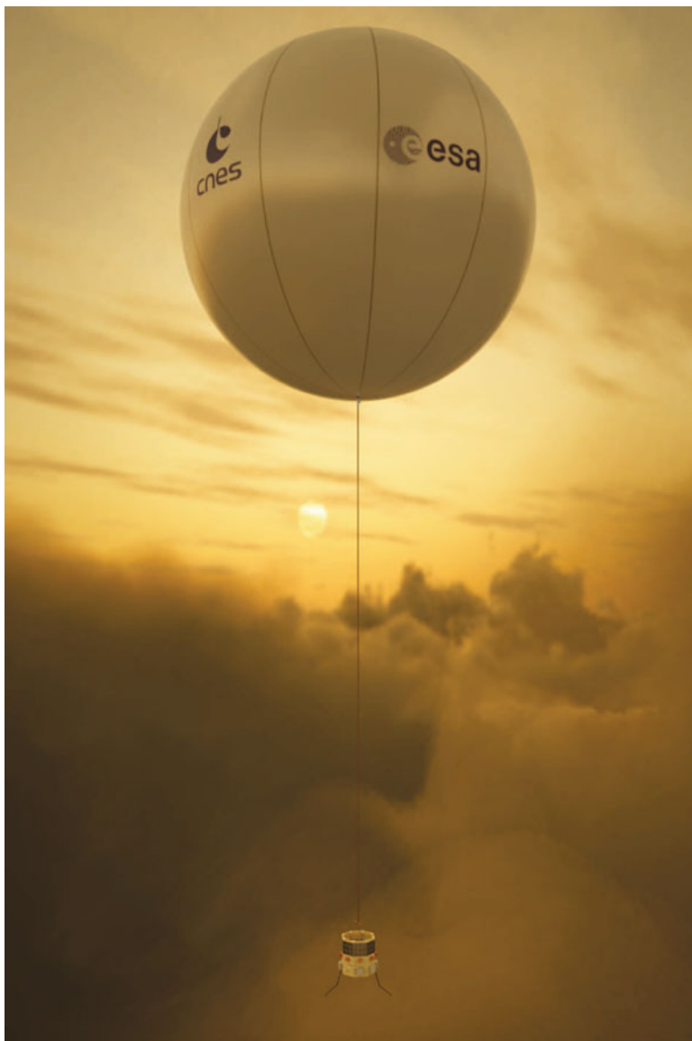
Fig. 10.4 An artist's impression of the European Venus Explorer, EVE. The helium filled super pressure balloon/gondola combination will float at 55 km altitude and will make at least one full revolution around the planet during its minimum lifetime of ten days. Courtesy of T. Balint, JPL/Univ. Paris-Sud/Univ. Oxford
