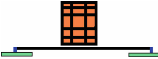
Fig. 9.4 Buckling of an elastic or rigid beam when weight is applied vertically
