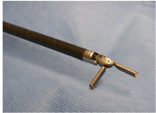
Fig. 4.6 Cobra grasper demonstrates the Cobra grasper used to manipulate the bladder to one side or another once it is mobile. This grasper is used almost exclusively in the third robotic arm. The tips can be very traumatic and we only use this on tissue that will be removed. This instrument should not be used to retract bowel
