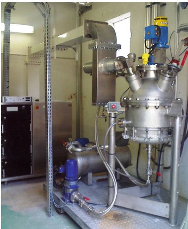
Fig. 8.5 Microwave-assisted batch reactor, 100 l. Installed microwave power 30 kW, 915 MHz. (Pilot installation at Ecole Nationale Supérieure de Montpellier, France)
