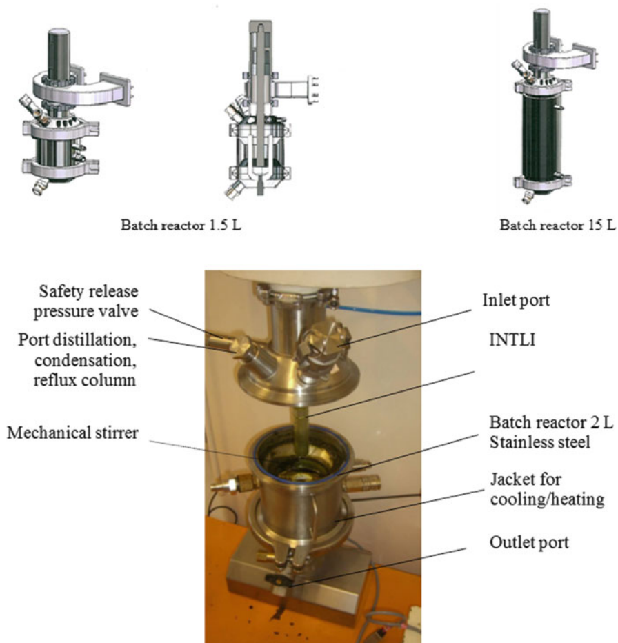
Fig. 8.3 LABOTRON extraction: batch reactors mounted on the U-guide
