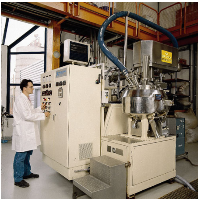
Fig. 3.9 Vacuum microwave hydrodistillation (VMHD) (100 l)
