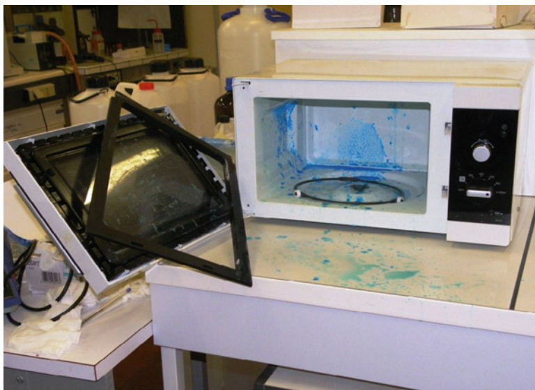
Fig. 8.10 Microwave oven after explosion in laboratory
