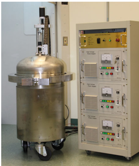
Fig. 1.7 UpScale Microwave batch-10 multimode reactor, fed by antennas. (Image from producer's commercial website: http://www.upscalemicrowave.com/ )
