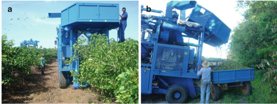
Fig. 5.10 Mechanical harvesting systems in physic nut from front (a) and lateral (b) (photos taken in Bioauto Farm, Nova Mutum, Mato Grosso, Brazil)
