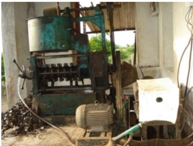
Fig. 19.1 Mechanical screw press for Jatropha cake production after oil extraction from seeds at a plantation (Chorvadla, Bhavnagar, Gujarat, India)
