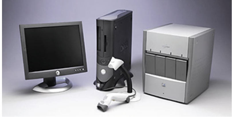
Fig. 14.15 GeneXpert ® Dx System. The GeneXpert ® instrument (right), shown with computer and barcode scanner. (Source: www.cephheid.com )
