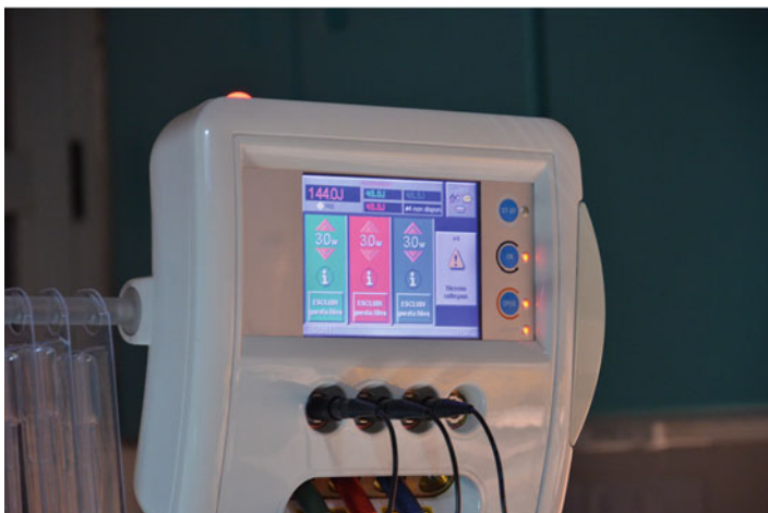
FIG. 13.12. The touch screen of the EcholaserX4® (Elesta, Florence, Italy) display permits the operator to use up to four sources each with its own activation and energy emission setting.
