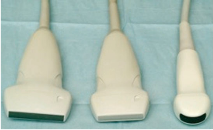
FIG. 12.1. From left to right demonstrates different footprint size, linear array transducers with the transducer on the right demonstrating a smaller, curvilinear array transducer.
