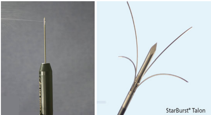
FIG. 13.26. Single tip ( left ) and multitined RF ( right ) electrode needles with tissue saline infusion reduce tissue desiccation with further ablation expansion.
