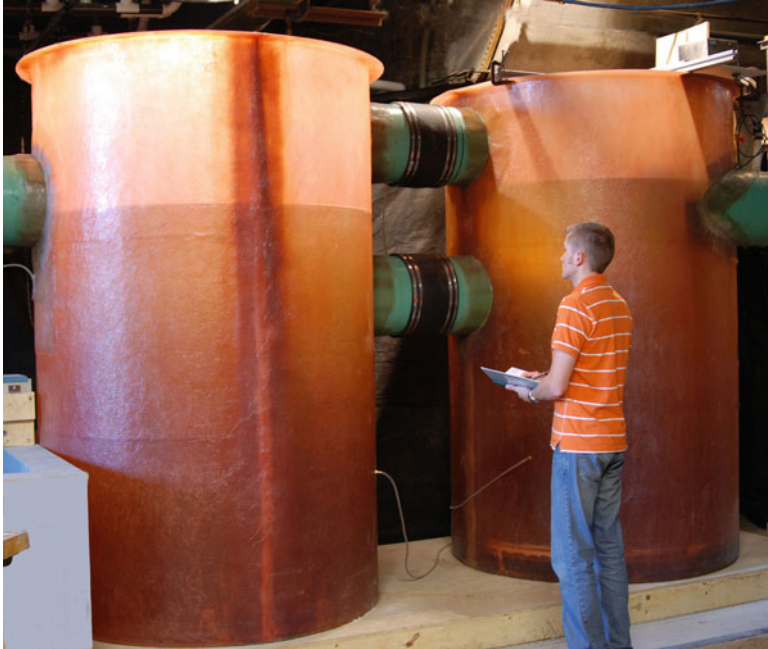
Fig. 4.3 Full-scale fiberglass prototype of a two-chamber hydrodynamic separator undergoing laboratory performance tests (Environment 21 V2B1 unit)
