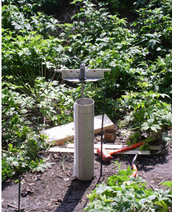
Fig. 6.4 Modified Philip-Dunne permeameter with ultrasonic sensor
